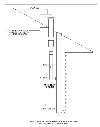
\*\*IMPORTANT NOTE: All vent pipes must be glued, properly supported, and the exhaust must be pitched a minimum of a 1/4" per foot back to the heater (to allow drainage of condensate).
